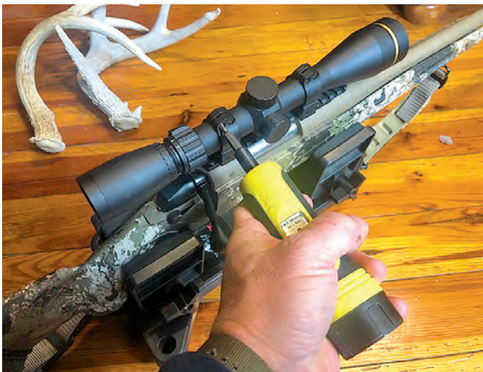
Tighten the rings only as much as the owner's manual suggests, and alternate tightening front and rear screws.
