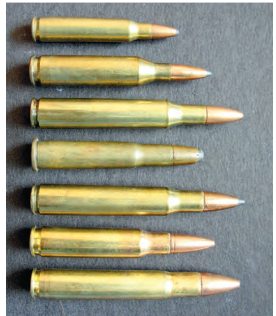
Whitetail cartridge comparison (top to bottom) .223 Rem, .243 Win, .270 Win, .30/30 Win, .30-06 Sprfld, .308 Rem, .35 Whelen.
