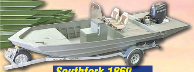
Southfork 1860 Fantail w/115HP, welded floor, 18 gallon fuel tank w/trailer
